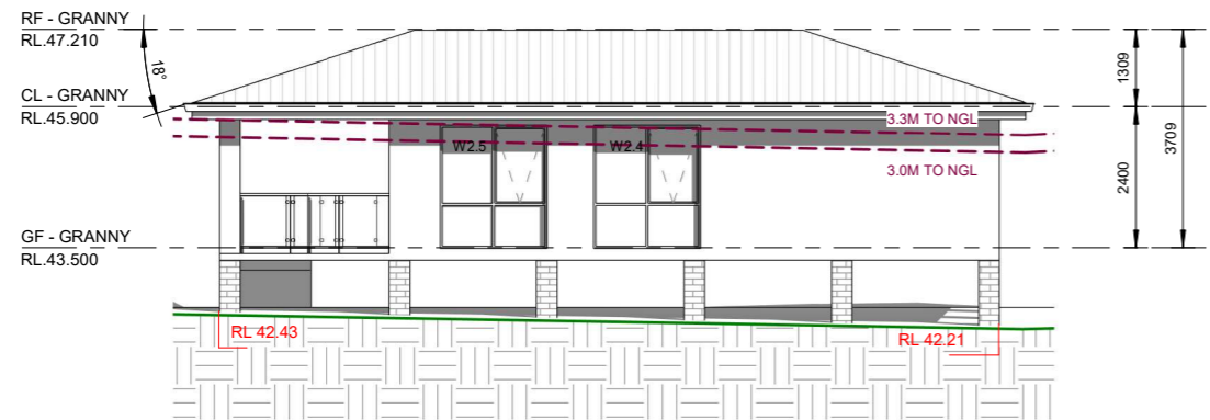
4 SOUTH EAST ELEVATION - GRANNY FLAT 1 : 100
